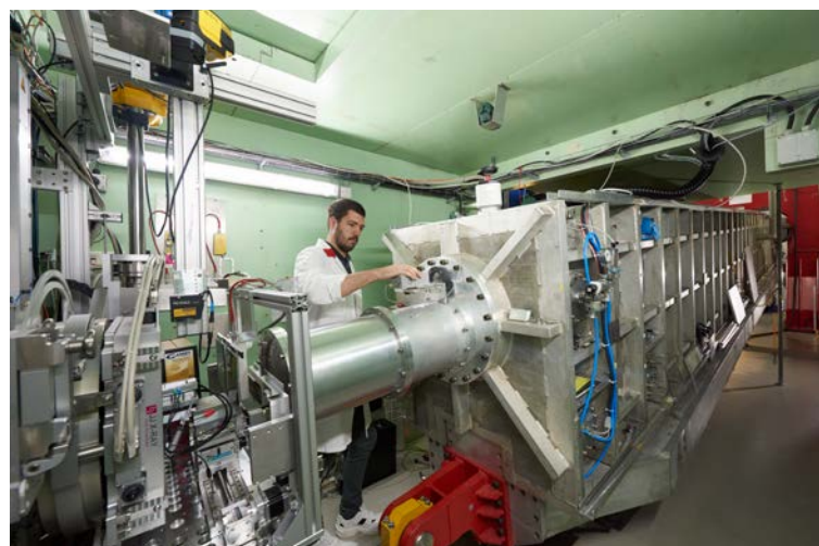
Fig. 1: The horizontal time-of-flight reflectometer with GISANS option REFSANS at MLZ.
