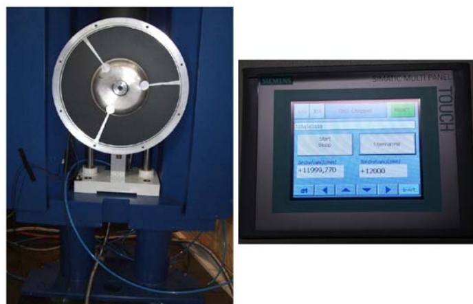
Fig. 1: DNS disc chopper system (left) and the chopper control panel that shows the chopper runs at 12 000 rpm (right).
