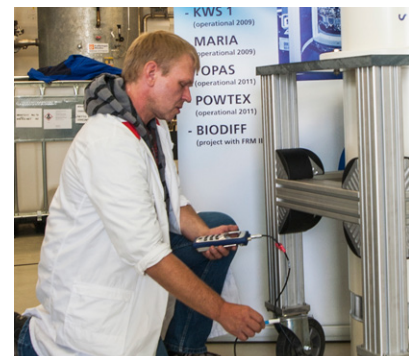
H. Schneider (JCNS) conducting the specification test of a 5 T cryomagnet.
