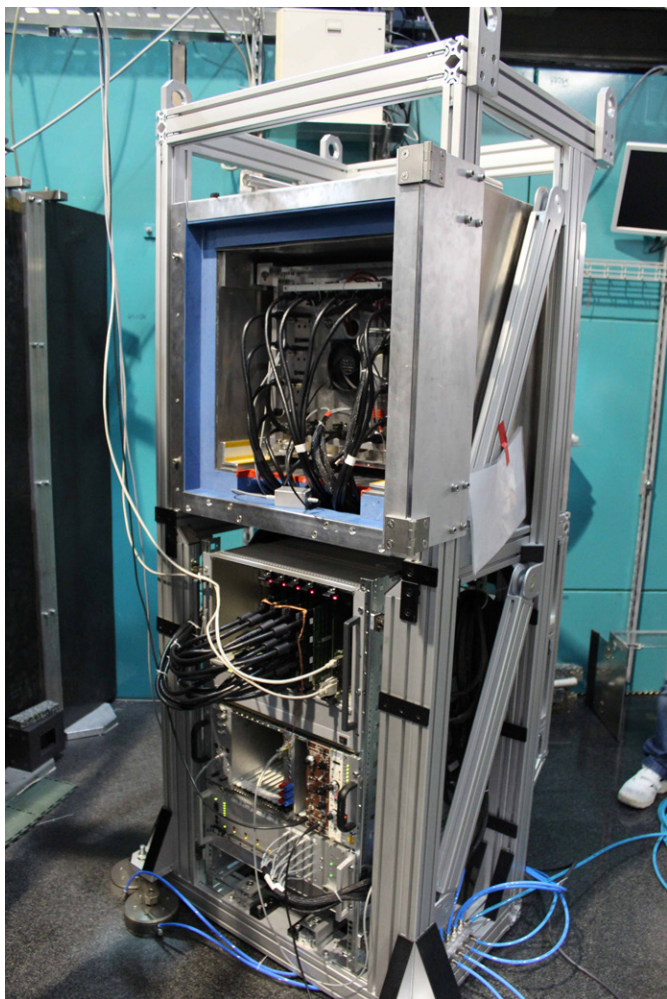
Fig. 1: New MWPC detector in its custom made housing including electronics.
