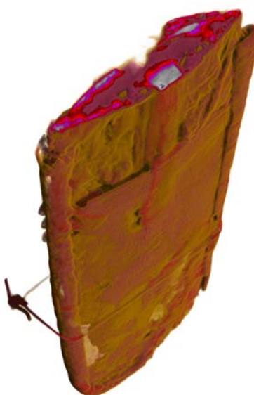
Fig. 2-3: Early medieval sword from Pforzen (Allgäu), 6 th century AD. The different layers of the scabbard can be clearly depicted by neutron tomography. A strip of wood was detected under the bronze metal sheet that covers the scabbard's front side.
