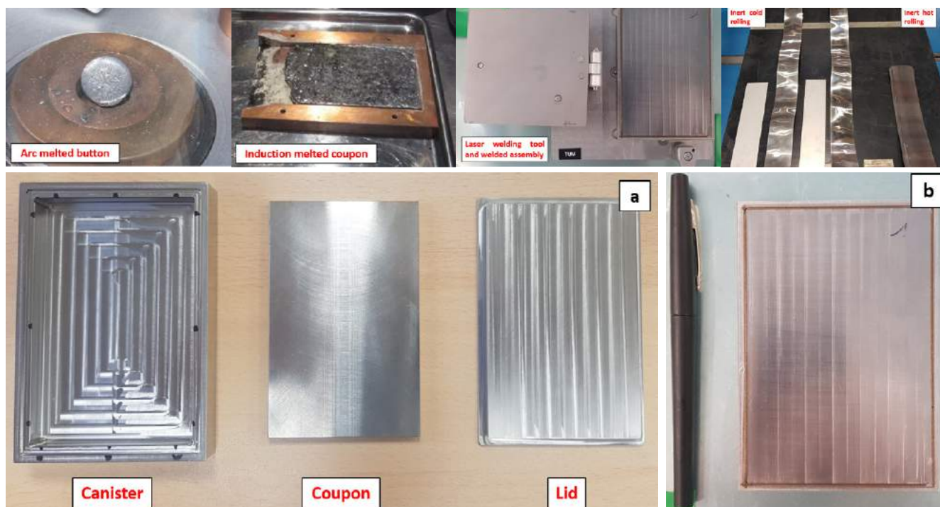
Fig. 2: Top: Different steps during the manufacturing process. Bottom: Assembly composition (a) and laser-welded assembly (b).
