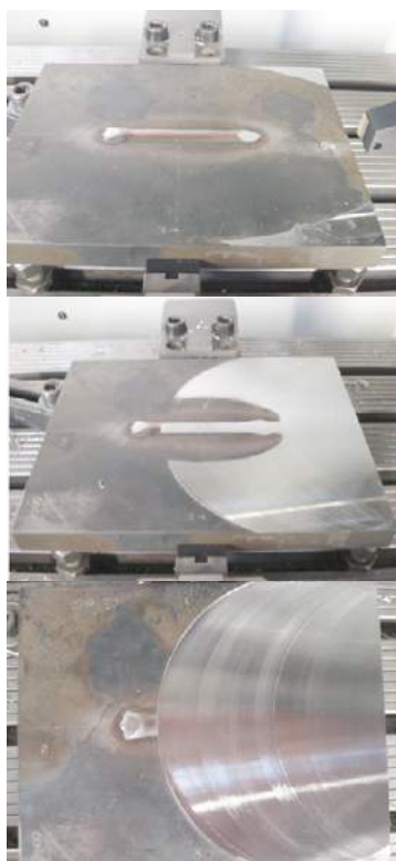
Fig. 1: Left: NeT-TG4, international benchmark weld plate after several passes of finish milling and by last machining state. Right: Residual stress profiles along the plate thickness for the as-welded (open symbols) and as-welded plus finish milling (full symbols) samples. Surface detail where comparison of longitudinal residual stress profiles, of the welded plus finish milling sample, measured by X-ray and neutron diffraction with finite element modelling, neutron spurious strain corrections and data deconvolution within the gauge volume are also pictured.
