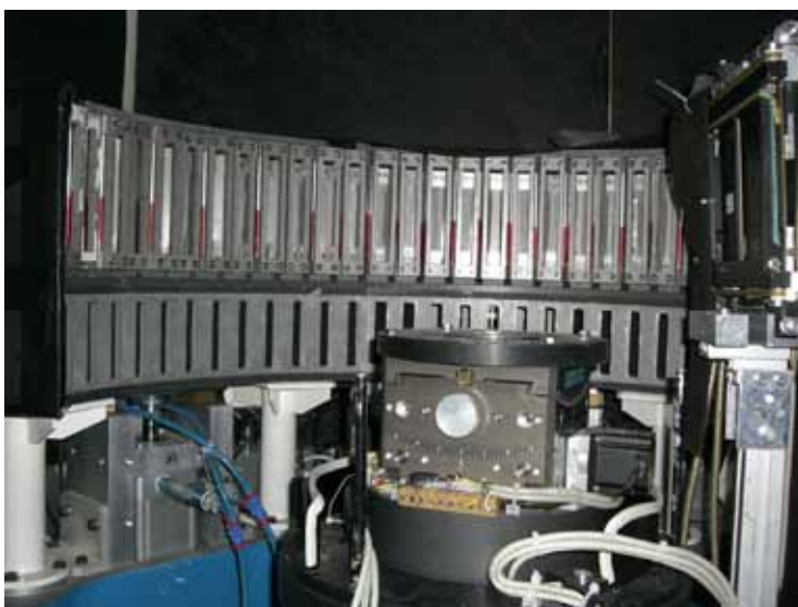
Fig. 2: Wide-angle polarization analyzers (24 units of m=3 supermirror benders).
