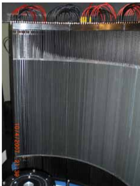
Fig. 3: New position-sensitive detector banks at DNS with 128 ^3\text{He} -tubes of 1m height and 0.5 inch diameter housed in a black radial collimation frame.
