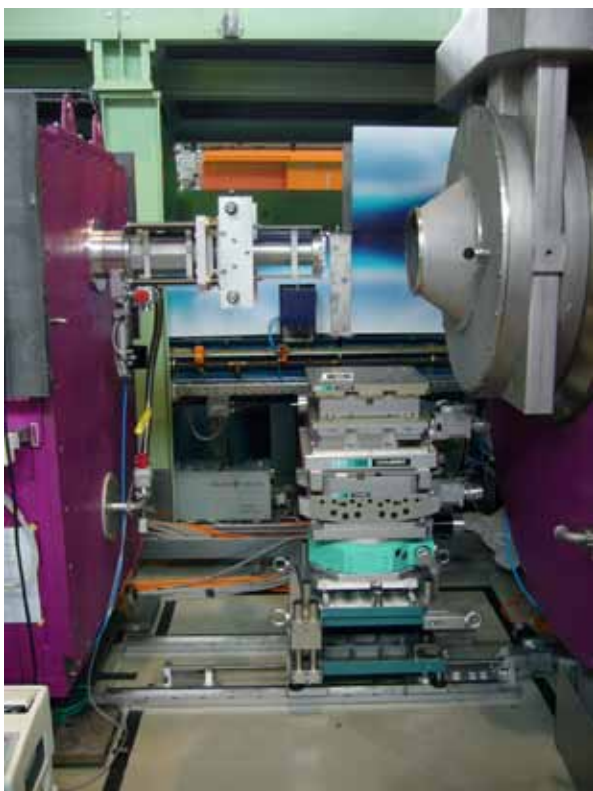
Fig. 4: The tower of sample environment for various set-ups
