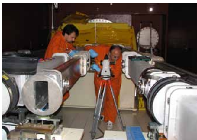
Fig. 4: Members of the neutron optics group aligning a new guide element in the neutron guide tunnel.
