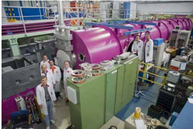
Fig. 1: The detector vessel and the end of the collimation part of SANS-1.
