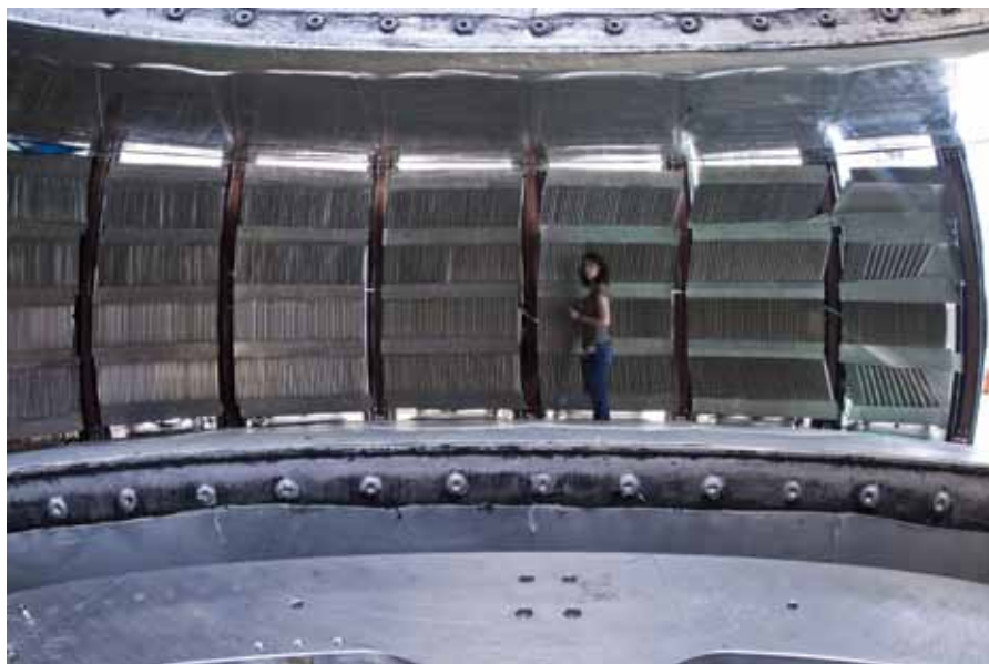
Dr. Giovanna Simeoni in the treasury room – view of the flight chamber from the sample position: 1006 ^3\text{He} detectors, aligned tangentially to the intersection lines between the Debye-Sherrer cones and the surface of a sphere (4 m radius) centered with the sample.
