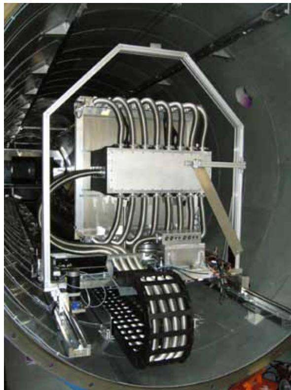
Fig. 5: The large area detector (backside) with electronic device in the detector vessel.
