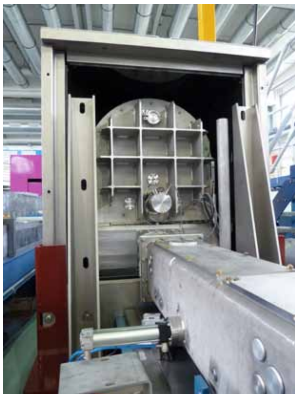
Fig. 1: The double-disc chopper installed in front of the collimation system; the chopper housing, the chopper shielding and the collimation housing with the pneumatic cylinder of the 20 th NG segment are visible.
