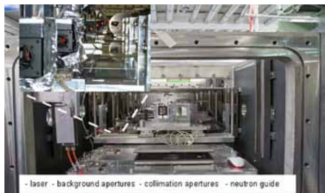
Fig. 3: A glance in the inner part of the collimation system with the four tracks marked in the photo.
