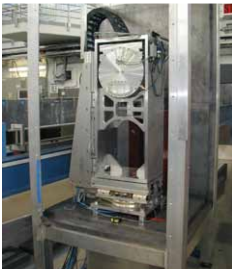
Fig. 2: The selector tower for flexible wavelength resolution and the possibility to provide a white beam for time of flight mode.
