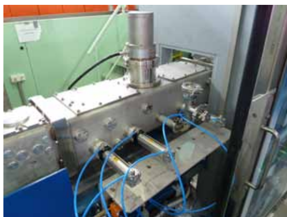
Fig. 2: The neutron lenses chamber; the cooling system and the pneumatic cylinders moving the three packages of \text{MgF}_2 lenses in and out of the beam are visible.
