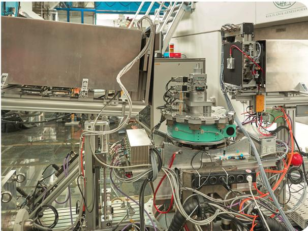
The neutron/ X-ray contrast reflectometer NREX, operated by the Max Planck Institute for Solid State Research, is designed for the determination of structural and magnetic properties of surfaces, interfaces, and thin film systems.
