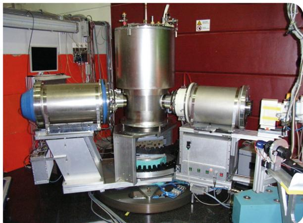
POLI is a versatile two axes single crystal diffractometer mostly dedicated to the investigation of magnetic structures in single crystals using neutron spin polarisation. The using of the separate non-polarising variably focussing monochromators and optimised polarisers allows the structural investigations using polarised and non-polarised neutrons with short wave length and high resolution. Two standard options are currently implemented on POLI:
