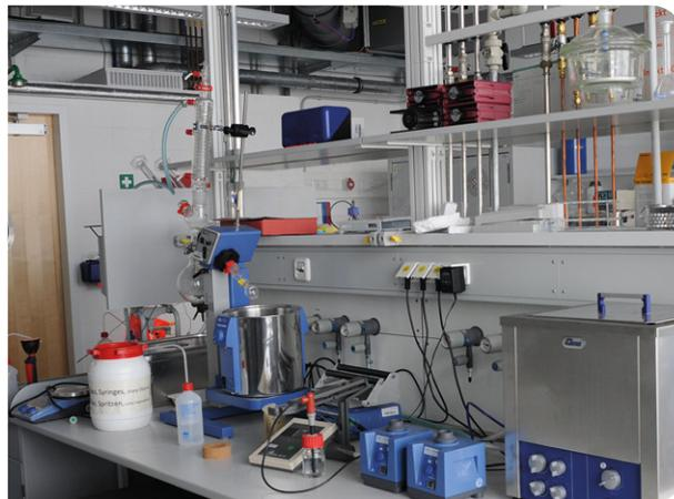
The chemistry and sample preparation laboratory is a 45 m<sup>2</sup> facility equipped with double hood to prepare samples for subsequent measurements on the neutron scattering instruments. It offers a basic tool set to handle samples from users, prepare solutions or even perform chemical reactions resulting in specific modifications. Samples can be handled under inert gas atmosphere like N<sub>2</sub> or Ar.
