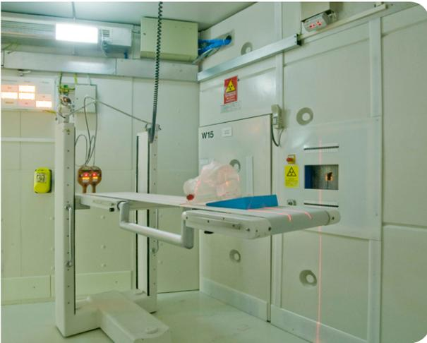
Figure 8: The tumour irradiation facility (MEDAPP) with a face mask for the accurate positioning of the patient. The Klinikum rechts der Isar (MRI), Department of Radiotherapy and Oncology, is responsible for conducting the therapy.
