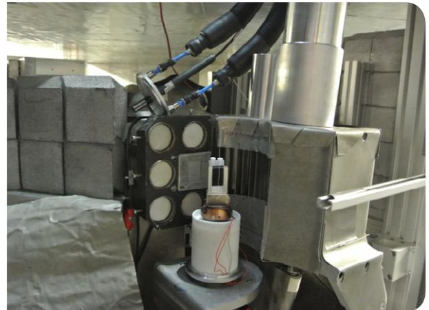
Measurement with customer cell at SPHERES on fuel-element parts.
