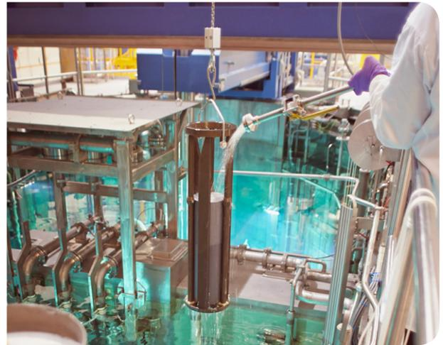
Figure 2: A freshly irradiated Si batch is taken out of the reactor pool.
