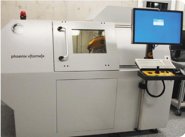
In order to offer an X-ray facility complementary to the neutron tomography station ANTARES, the FRM II and the Chair of Biomedical Physics at the TUM have started to operate a high resolution computer tomography facility. The “micro CT VtomeX” is also available to users of the MLZ. Samples, that can be examined, include geo and composite materials, semiconductors and biomedical specimens.
