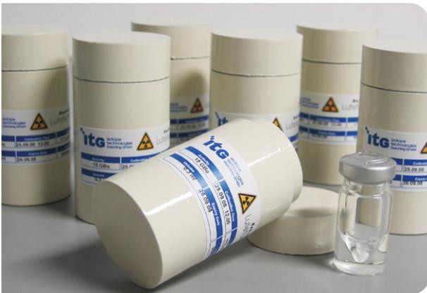
Figure 6:  $^{177}\text{Lu}$  produced by the company ITG at the FRM II at the capsule irradiation facility. The radioisotope is filled in little vials with a volume of 2 ml and then packed in cans with a diameter of 45 mm and a height of 70 mm.
