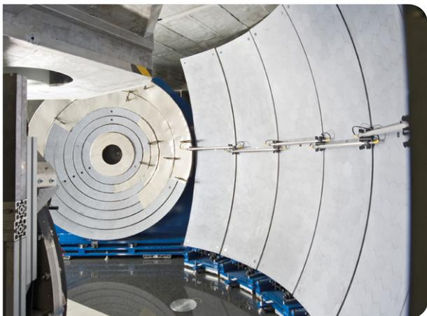
SPHERES (**s**pectrometer for high energy **r**esolution) is a third-generation backscattering instrument with focussing optics and a phase-space-transform chopper. It is a versatile spectrometer for the investigation of atomic and molecular dynamics on a GHz scale.
