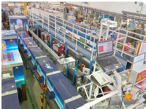
KWS-3 is a very small angle neutron scattering (VSANS) instrument running on the focussing mirror principle. The principle of this instrument is a one-to-one image of an entrance aperture onto a 2D position sensitive detector by neutron reflection from a double-focussing toroidal mirror.
