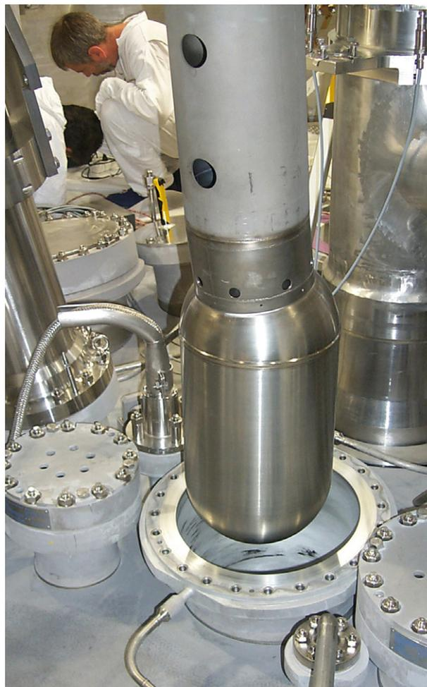
Figure 3: The moderator of the hot source in the reactor pool of the FRM II during installation.
