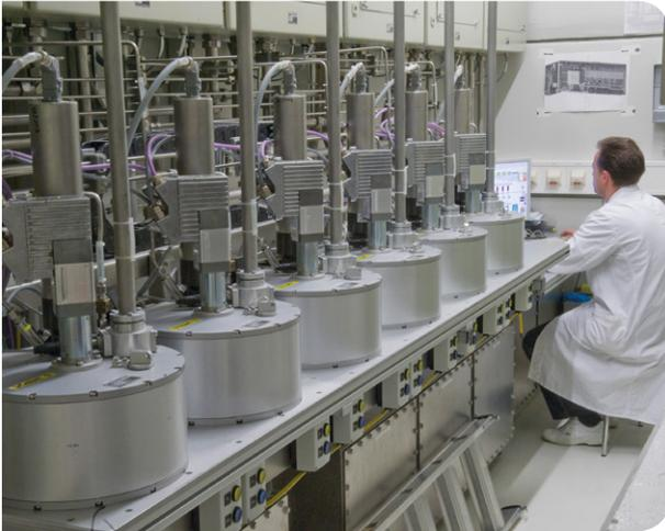
Figure 3: The standard rabbit irradiation system has six independent irradiation channels and is operated by carbon-dioxide.
