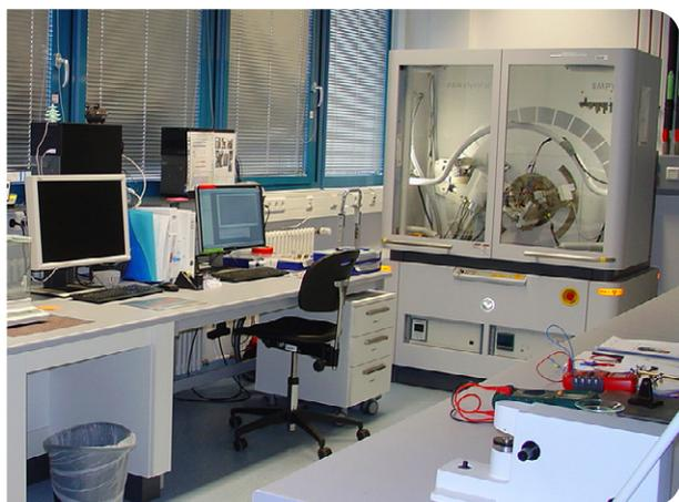
In collaboration with HZG and TUM, the Materials Science Lab serves as laboratory to prepare samples (polishing, cutting, etching, and annealing) for subsequent neutron scattering measurements. It is equipped with several analytic instruments for instance X-ray Diffractometer (XRD) mainly for battery research and high-performance materials, Differential Scanning Calorimeter (DSC), Micro-Hardness and Optical Microscopes to perform complementary analytics.
