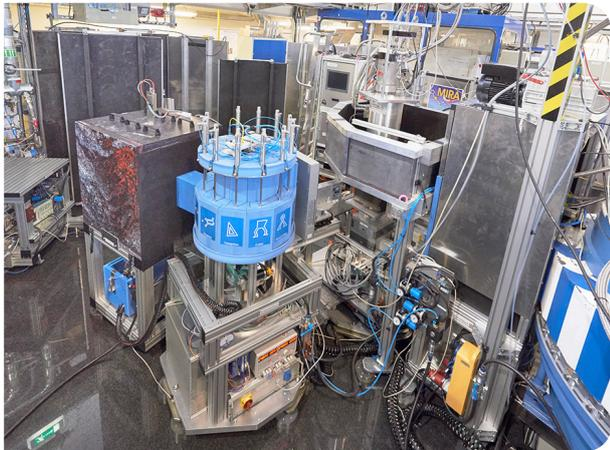
MIRA is a multipurpose instrument. With its two beam ports, namely MIRA-1 and MIRA-2, it provides neutrons over a wide range of wavelengths  $3.5 \text{ \AA} < \lambda < 20 \text{ \AA}$ . The instrument can easily be moved from one port to the other without changing the sample environment. The large variety of different options offered can also be combined in most cases. This allows for a fast realisation of experiments in a very flexible way using a number of available options:
