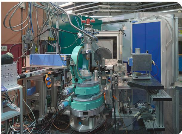
The diffractometer RESI is designed for using a maximum of thermal neutron intensity, allowing optimum measurements of weak diffraction phenomena in a large portion of the reciprocal space on single crystalline samples.
