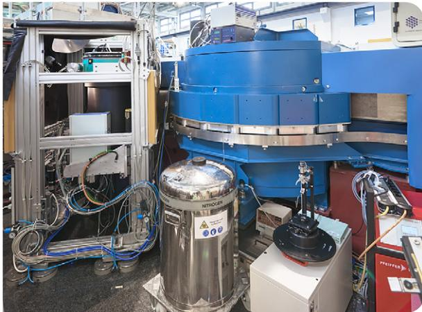
The monochromatic single crystal diffractometer BIODIFF is a joint project of the FRM II (TUM) and JCNS (Forschungszentrum Jülich).
