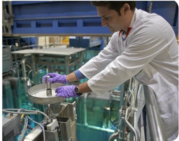
Figure 7: Loading of the capsule irradiation facility.
