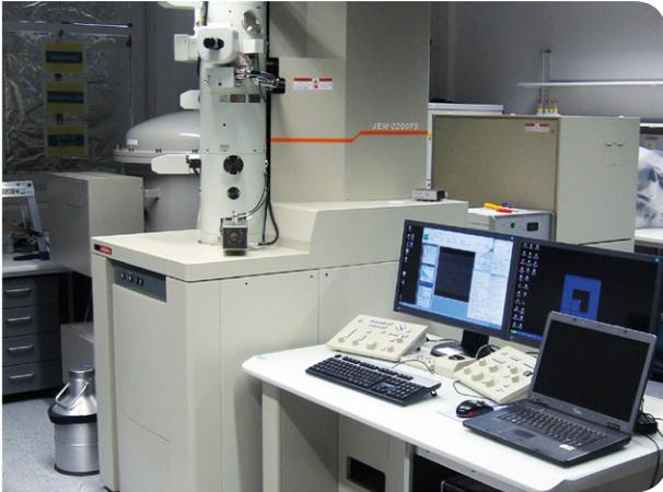
Transmission electron microscopy is a complementary technique with neutron scattering in the frame of soft matter studies. With the TEM, real space investigations are performed to access information about shape, size, and size distribution of particles, self-assembly and aggregation. Users will be supported by JCNS staff (M.S. Appavou) to conduct the suitable preparation and TEM investigation.
