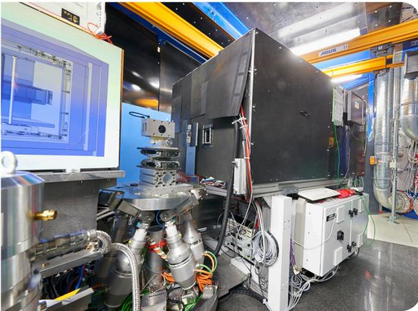
The neutron reflectometer MARIA with polarisation analysis was designed for the investigation of thin magnetic layered structures down to the monolayer scale and lateral structures. The reflection of polarised neutrons allows to determine individually the density and the modulus and the direction of the magnetisation vector of buried layers.
