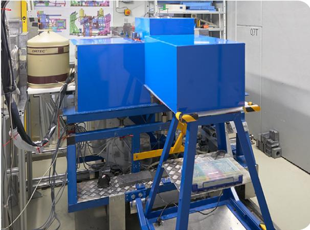
Prompt gamma-ray activation analysis (PGAA) is typically used for the determination of elemental composition and concentration of solid samples (ca. down to ppm range). Liquids and gaseous samples can also be measured.
