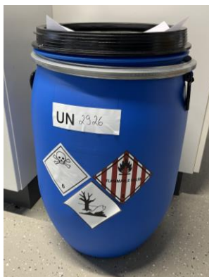
blue bin for chemically contaminated equipment e.g. empty bottles, gloves, paper wipes
