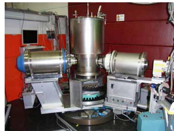
Figure 3: POLI-HEiDi with the new CRYOPAD installed.
