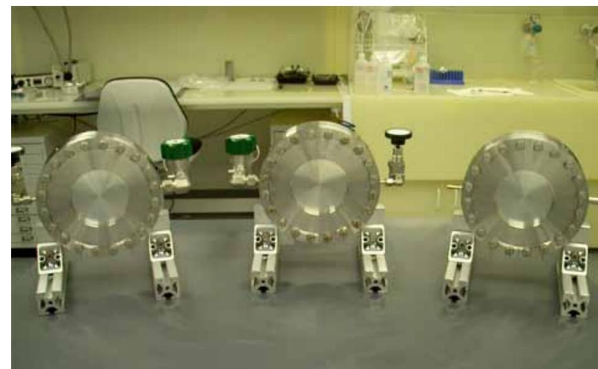
Figure 2: Test detectors for developing Gaseous Scintillation Proportional Counters.
