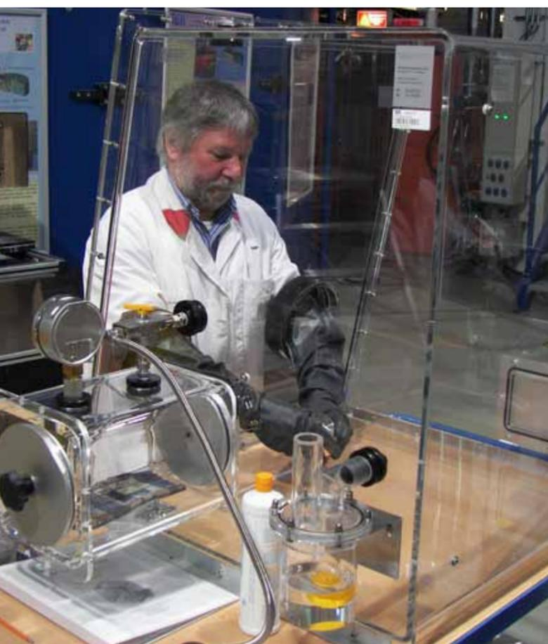
Figure 4: New mobile glove boxes available in the experimental areas.
