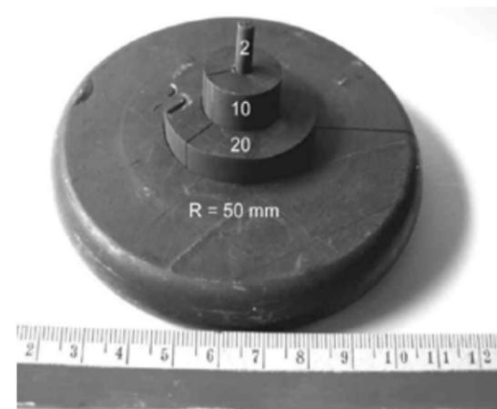
Figure 1: Photography of the disc after the experiment. The disc radii were reduced stepwise by electrical discharge machining. The results for the discs with radii of 10 and 20 mm are discussed elsewhere.
