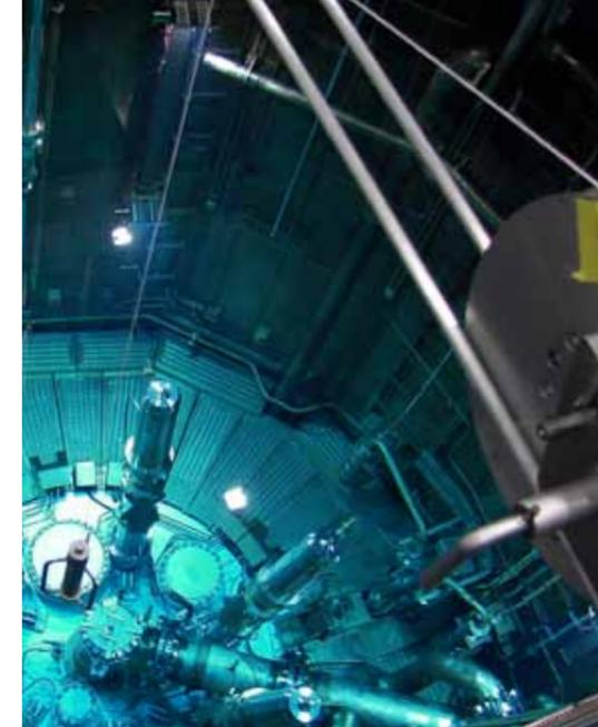
Figure 2: The high volume irradiation facility at the FRM II reactor pool, which is used to identify the age of rock.
