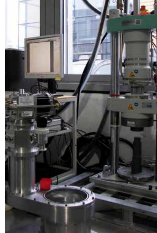
Figure 3: Liquid-cooling free cryostat (front) to be mounted in the high pressure machine (back).
