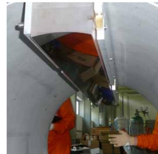
Figure 2: The new double focussing mirror of KWS 3.
