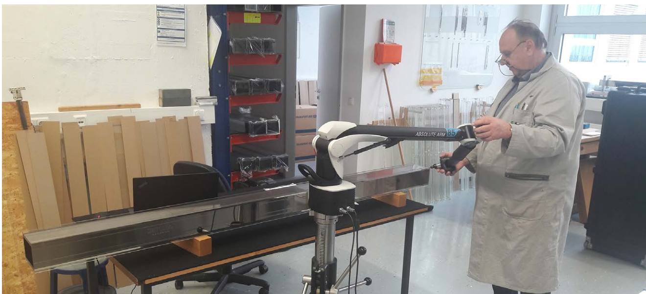
Figure 7: Our new Romer Absolute Arm 85 in action. The portable device has an access area of up to 2m diameter, an ideally suited high precision instrument component survey and fiducialisation. Here, a neutron guide element is the object of geometrical control after assembly.
