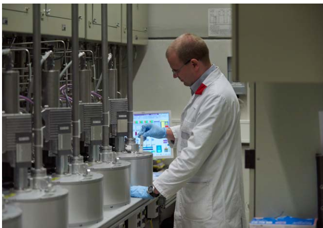
Figure 1: Florian Jeschke - head of the irradiation facilities - inserts samples into the pneumatic delivery system of the FRM II.
