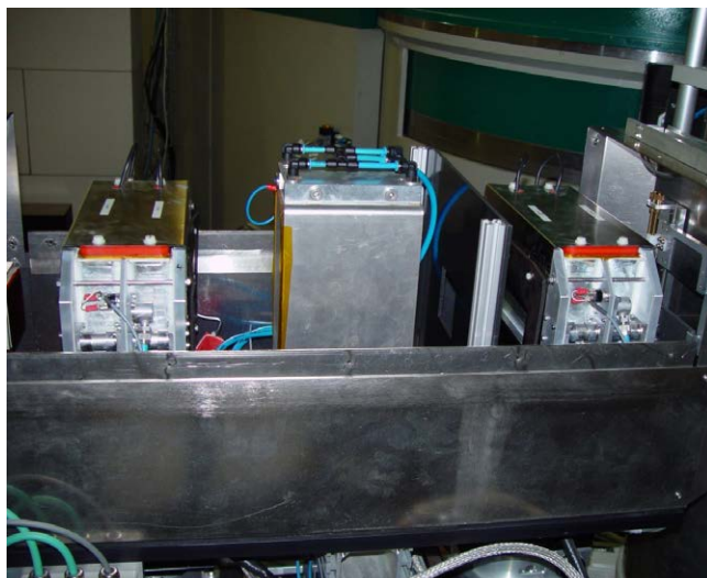
Figure 7: DC coil (center) in between two RF spin-flippers at TRISP. The coil generates a vertical field of about 150 Gauss and is surrounded by a mu-metal yoke to avoid stray fields. The winding is made from pure aluminum wire (diameter 1 mm). Insulation is achieved by 0.1 mm gaps between the turns of the winding.
