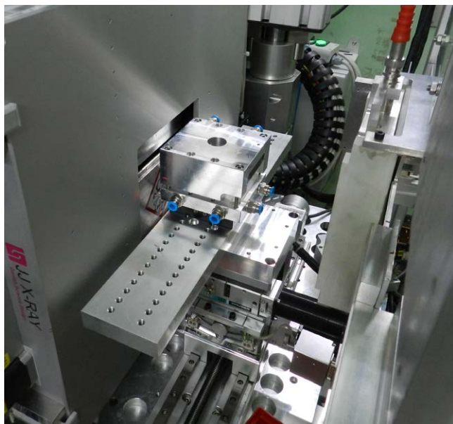
Figure 2: A cell for the study of liquid/solid interfaces installed at Refsans. In order to optimise the sample illumination, the cell is placed at the shortest possible distance from the last slit. A magnetic sample holder ensuring rapid and accurate repositioning makes cell changes a breeze. The round hole in the top of the cell is a viewport to the silicon wafer and is being used for accurate optical alignment by means of an autocollimator.
