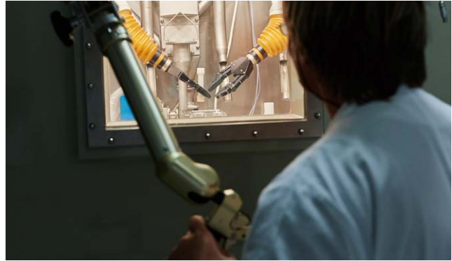
Figure 2: An operator handles the sample after irradiation by means of a manipulator.
