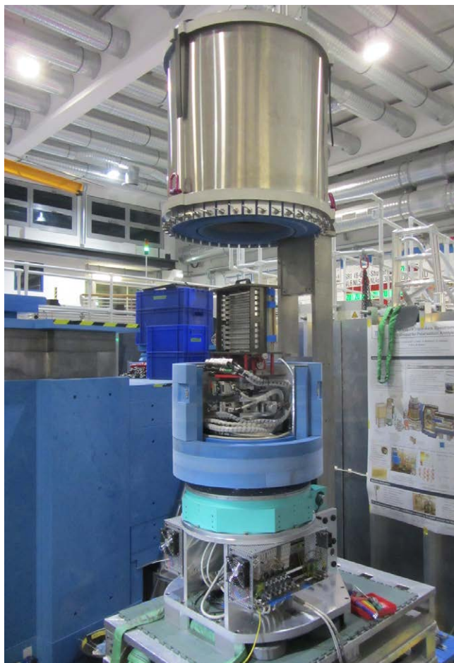
Figure 1: Fully assembled analyser-tower prepared for commissioning at the instrument. The neutron-absorbing borated polyethylene shielding blocks are fixed in the upper position and a side door is opened to show the positioning and focusing mechanics and the corresponding cabling.
