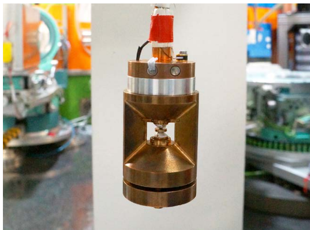
Figure 1: The panoramic diamond anvil cell used for the high-pressure neutron single-crystal diffraction measurements.
