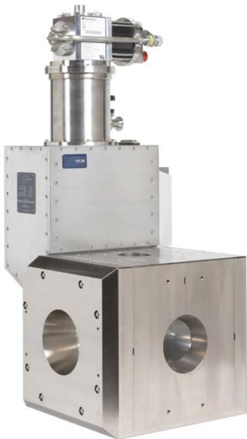
Fig. 2: The brand-new 3 T magnet for the SANS instruments.
