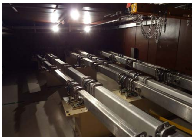
Fig. 1: Neutron guide tunnel with the neutron guides inside the vacuum housings. NL1 to NL6 from left to right.
