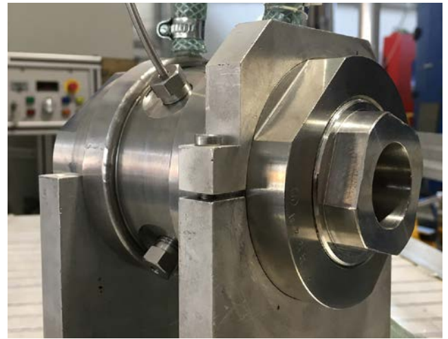
Fig. 1: The T1001plus gas pressure cell with sapphire windows (top).
