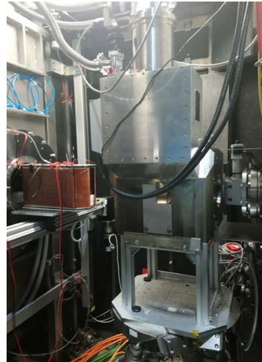
Fig. 3: The 3 T SANS magnet on top of the hexapod at KWS-1 (field direction is parallel to the neutron beam). To the left the magnetic cavity for the ^3\text{He} analyzer is seen.
