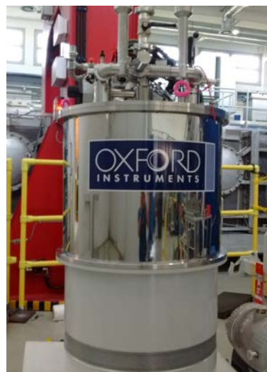
Fig. 1: The impressive 12 T magnet for diffraction and spectroscopy
