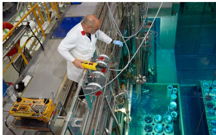
Workplace at the cooling pond: Operator J. Molch rearranges the Si-crystals into the irradiation baskets.
