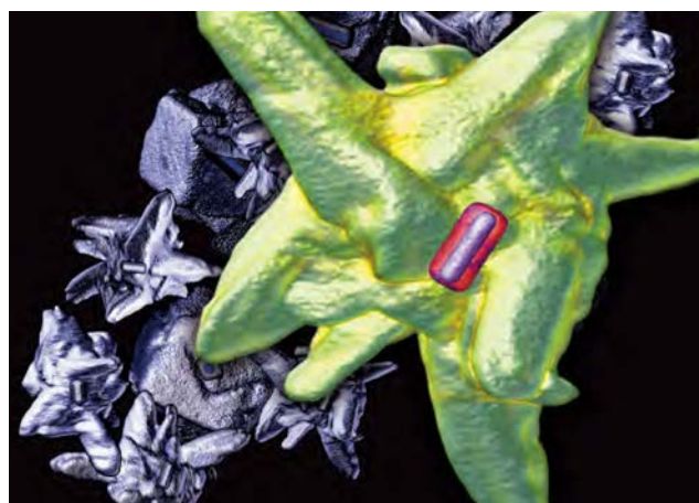
3D visualisation of an electron tomography reconstruction of a Ag/Au nanorod encapsulated by a MOF. Sample courtesy: I. Pastoriza-Santos, J. Perez-Juste (University of Vigo).
