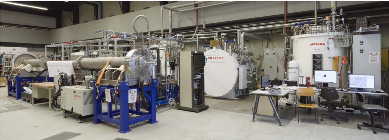
Fig. 3: Left: A 1:1 rebuild of the SR6 beam tube of the FRM II. Right: The control station of the test set-up. Back: The cold boxes of the cooling system.
