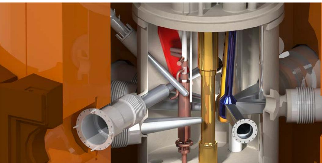
Fig. 1: The compact core concept of FRM II: View into the  $D_2O$  moderator tank. The fuel element is located in the central channel (gold), surrounded by beam tubes (grey), secondary sources (red: converter facility for fast neutrons, blue: cold source) and safety and measurement installations (not all components are shown).
