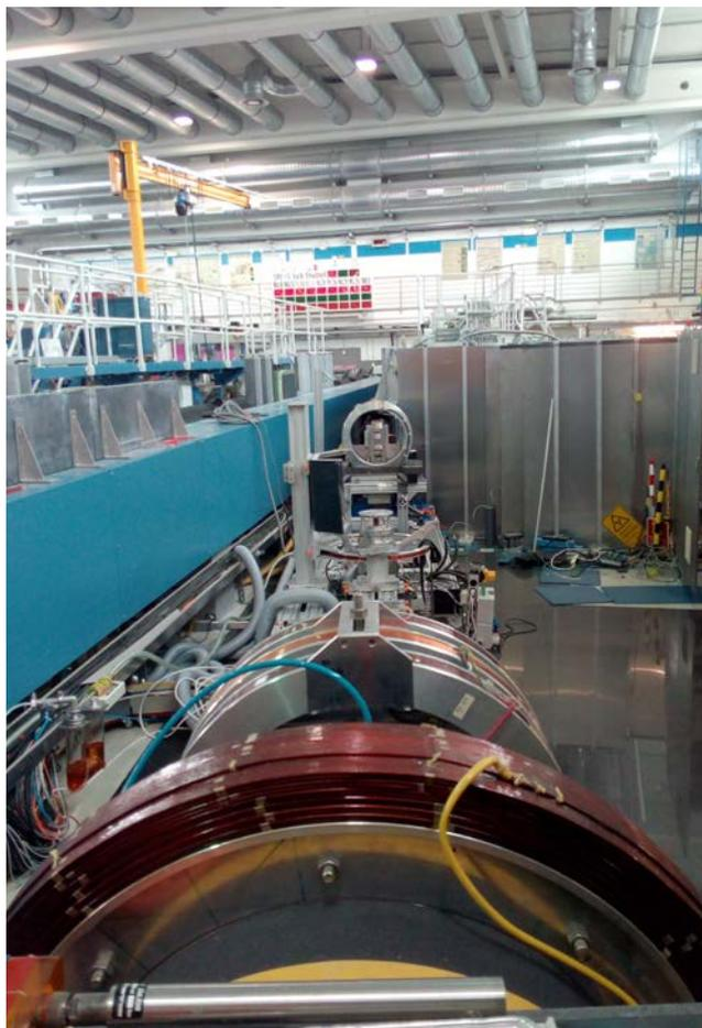
Fig. 2: Empty carriers, after the main coils have been removed, waiting for the cool superconducting solenoids.
