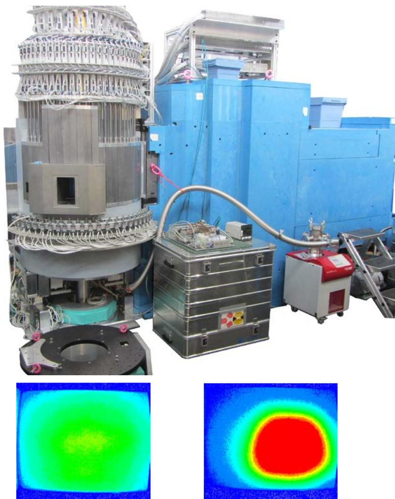
Upper panel: photo of the beamline KOMPASS. Bottom panel: Images as acquired using a neutron camera for the monochromator in the flat (left) and doubly focussing configuration (right).
