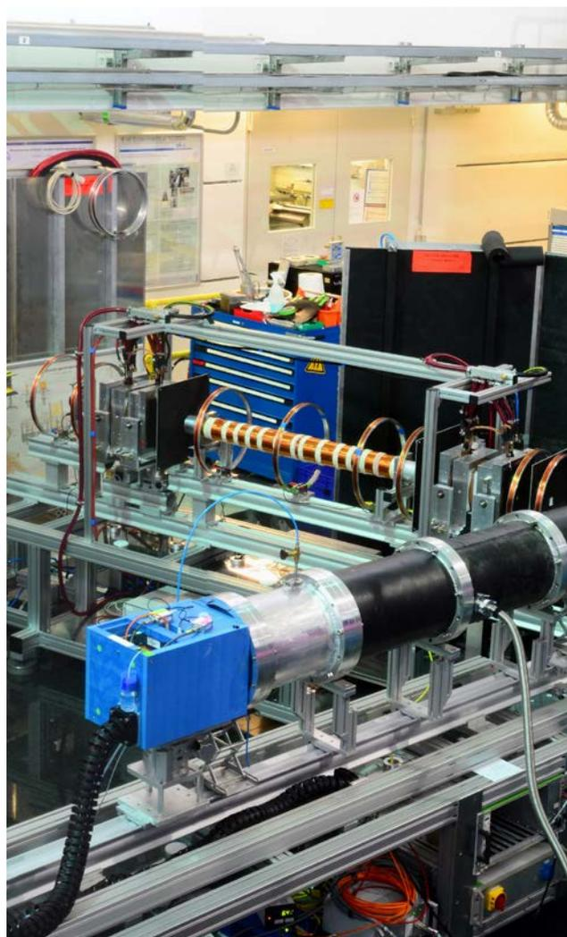
Fig. 3: Secondary spectrometer arms of RESEDA, NRSE arm with black detector box, MIEZE arm with CASCADE detector in the blue shielding box.
