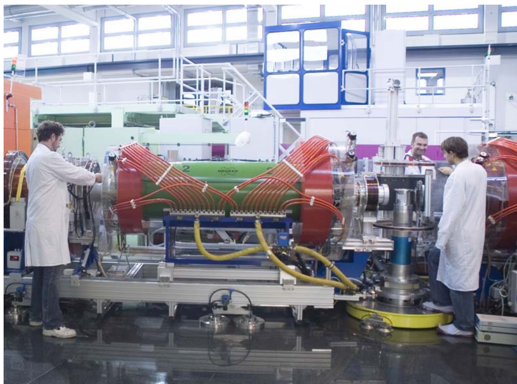
Fig. 1: Sample stage and second arm of the J-NSE spectrometer with the main precession coil (green).
