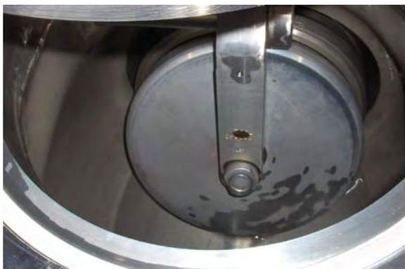
Figure 1: The main check valve to which a second, new one has been added.
