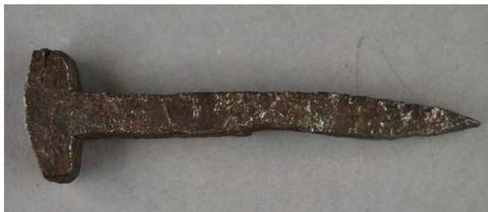
Figure 3: A Celtic nail from the oppidum of Manching (ca. 9 cm long) containing only 37 ppm of Cl after thermal treatment in welding gas (N<sub>2</sub> + 10 % H<sub>2</sub>) at 750 °C. The treatment took place 25 years ago and the nail survived with hardly any corrosion. PGAA shows that it contains only 37 ppm of chlorine.
