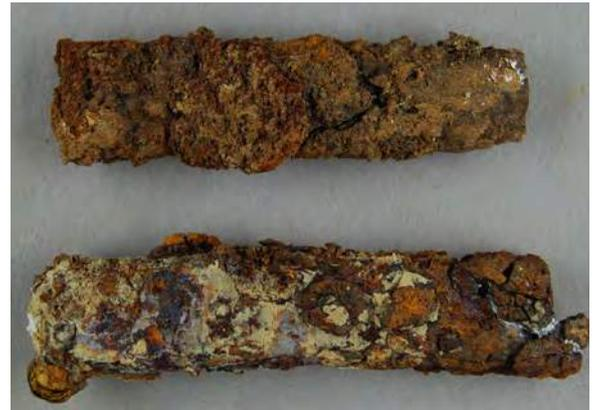
Figure 2: Two heavily corroded iron strap ends (about 8 cm long) used to protect the ends of leather straps from the same grave excavated at Steinheim near Dillingen (Bavaria) in 1996. The upper piece is untreated, the lower one was leached in an alkaline solution of  $\text{Na}_2\text{SO}_3$  for three months. They look very similar, but the unleached one contains 1300 ppm of Cl, while the leached one contains only 110 ppm.
