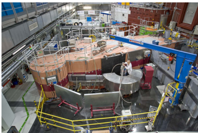
Figure 2.2.: At the structure powder diffractometer SPODI lithium-ion batteries and hydrogen storage materials have been studied.
