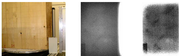
Figure 4.27.: Penetration of 49.2 cm wood with an additional Lucite block as a contrast giving body (positioned between wood specimen and the detector screen, photo left). Centre: Sum of filtered raw images. Right: Image after median filtering and correction for the open beam intensity distribution (structural details of the wood becoming visible).
