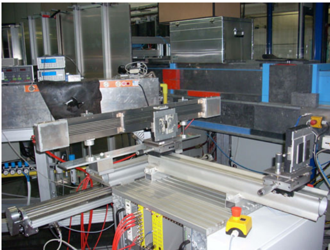
Figure 1.7.: SANS1 prototype detector consisting of 8 PSDs mounted on the x-y scanning table of the new detector test beam station at TREFF .
