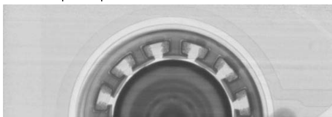
Figure 4.10.: Normalized high-resolution radiograph recorded with the periscope at L/D=800 at ANTARES.
