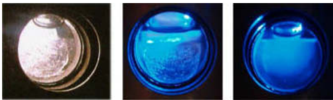
Figure 5.11.: Melting of the gas crystal as a function of time \sim 10 min at T_{cell} = 22 K. The crystal melts in vertical layers and from the top.
