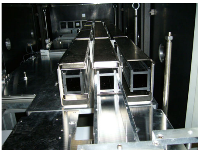
Figure 2.8.: Two polarisers (left and middle) and one neutron guide Ni^{58} (right) are mounted on a moveable table. U-shaped support of soft iron is used to mount permanent magnets.
