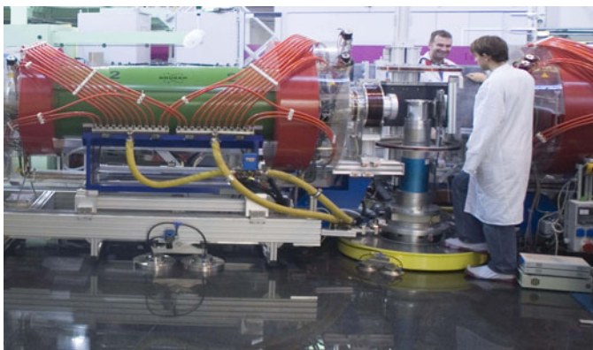
Figure 3.11.: The sample position (on the right) and second precession coil (green) of the J-NSE spectrometer.
