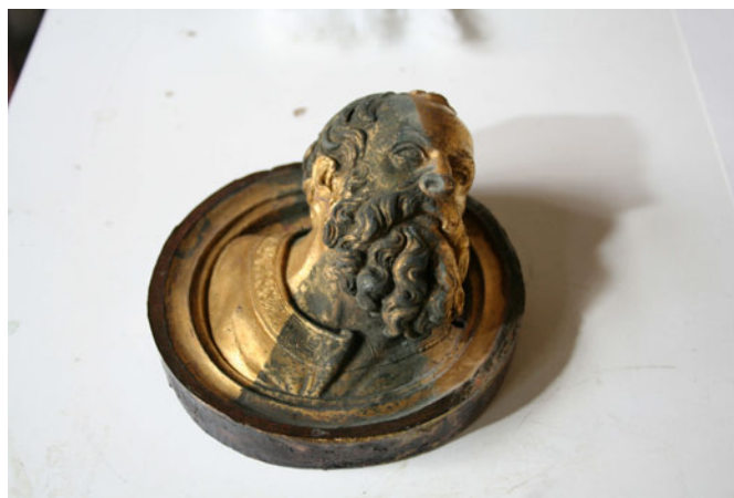
Figure 4.2.: Head of the prophet of Lorenzo Ghiberti made of gilded bronze. It is part of the "Paradise Gate" of the Baptistery of Florence, Opera di Santa Maria del Fiore. The left part was cleaned with a laser technique and the right one with a wet chemistry method (Rochelle salts). The middle part is still uncleaned.
