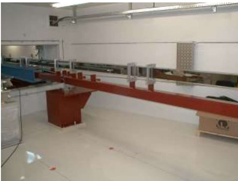
Figure 8.9: The NG NL6 entering the NG hall. Shown are the supporting construction of the neutron line and the optical elements with their adjustment frames. The final lead cover has not yet been mounted.
