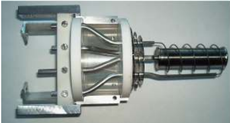
Figure 5.1: The opened (i. e. without heat shields) MAFF ion source prototype.
