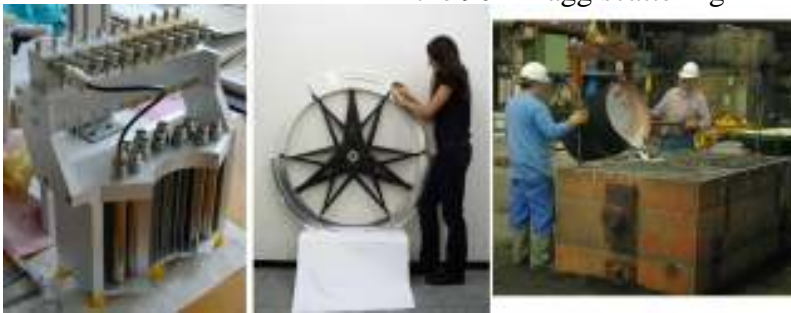
Figure 4.12: left: Detector bank (finished in 2001). Centre: Chopper wheel with crystal support dummies. Right: Casting of large angle analyzers at Mittelrheinische Gießerei, Andernach.
