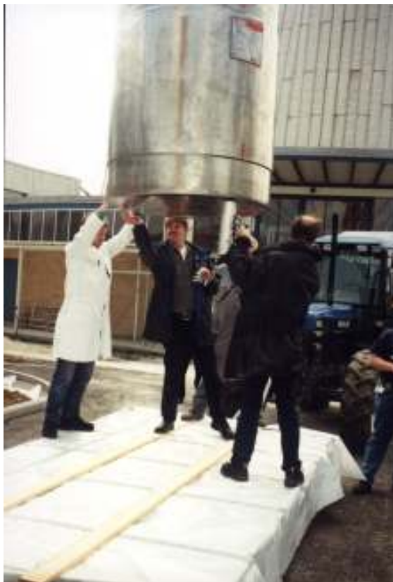
Figure 9.1: Loaded transport cask filled with water for shielding purposes.
