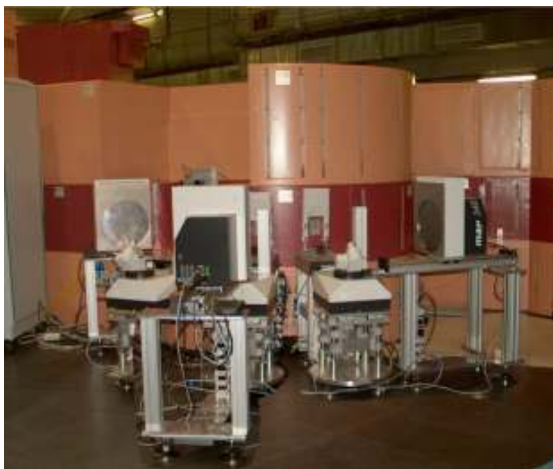
Figure 3.6: View of the secondary diffractometer. This image shows three different configurations of the goniometer.
