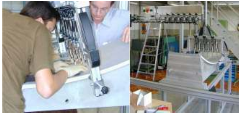
Figure 4.17: Fixing of Si(111) crystals on a large angle analyzer.
