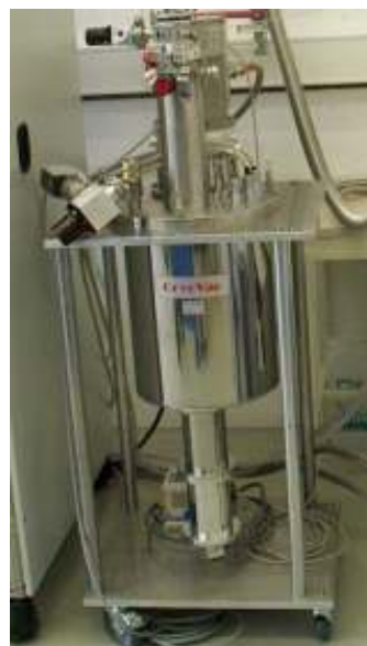
Figure 8.4: Cryogen Free Sample Tube Refrigerator
