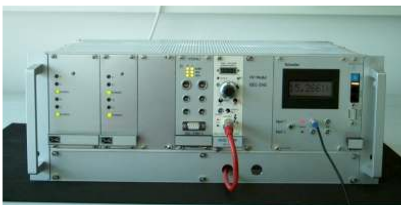
Figure 8.2: Remote controlled Bias and HV-power supply system with ratemeter for ^3\text{He} - and monitor detectors
