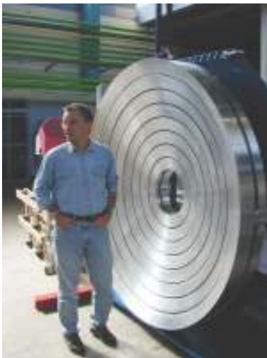
Figure 4.16: Debye-Scherrer rings before glueing of the Si(111) crystals.
