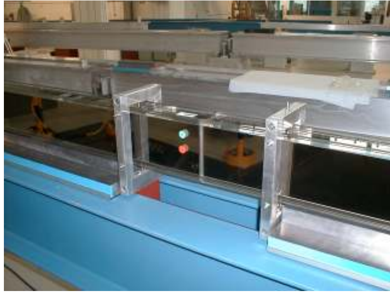
Figure 8.10: Details of the NG NL6. The figure shows the joint of two optical elements with the corresponding adjustment frames. Between optical elements and the mechanical support the bottom lead shields have been introduced.
