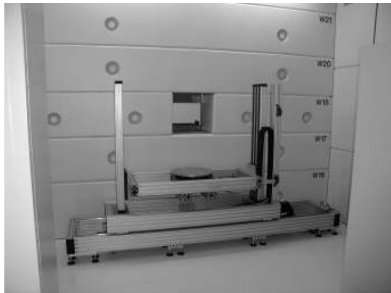
Figure 6.11: Manipulator at measuring position at the converter facility.
