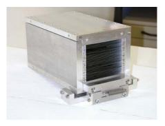
Figure 2.21: The polarisation analyzer of TREFF.
