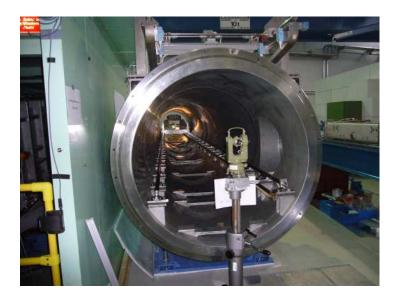
Figure 2.2: Inside view of the KWS-2 detector housing.
