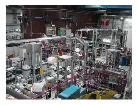
Figure 7.1: The positron beam facility NEPOMUC and positron spectrometers in the experimental hall of FRM II: CDB spectrometer (TUM), PAES-facility (TUM, not shown), apparatus for Ps<sup>-</sup>-production (MPI nuclear physics, Heidelberg), and components of the pulsed-beam facility PLEPS (UniBW, Munich).
