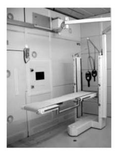
Figure 8.5: Medical irradiation room with treatment couch. The fixed horizontal beam enters from left, 1.45 m above the floor.
