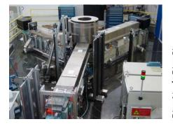
Figure 4.5: The instrument RESEDA with its two secondary spectrometer arms. The mu-metal shielding of the left arm is removed and gives free view on the NSE and NRSE coils.
