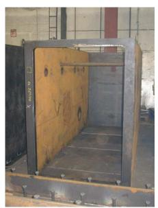
Figure 2.19: Vacuum chamber.
