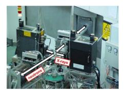
Figure 2.12: The N-REX<sup>+</sup> sample table with compact X-ray source and detector units mounted for simultaneous neutron/Xray reflectivity experiments. The neutrons are impinging from the monochromator hutch on the right, the neutron area detector (not shown) is located on the left.
