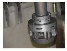
Figure 8.3: new design of the coupler for the sample container.
