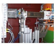
Figure 3.9: Magnetostatic cavity MB2 fixed on the rotating flange permitting 180° "flipping"
