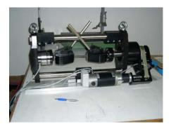
Figure 3.16: 50 kN load frame with grips for flat samples attached.
