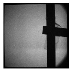
Figure 6.5: The cold source at 3 MW with the Figure 6.7: The cold source at 3 MW with polethylen strips in the beam, with the geometric center marked by the upper corner of the horizontal strip.
