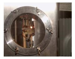
Figure 9.12: Electromagnetically levitated liquid Ni droplet at a temperature of 1810 K. The water cooled copper coil is shielded with a neutron absorbing rubber. The radial collimator of Tof-Tof is on the right.
