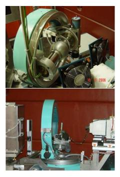
Figure 3.4: Large (top) and small (bottom) furnace in Eulerian cradle
