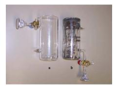
Figure 3.7: a) Spin filter cell *Heidi2*: Small metallic Cs droplets in the lower part of the cell and in the appendix are visible; b) Cell *Heidi1*: The dark spots inside the cell are traces of Cs sub-oxide which is liquid at room temperature.
