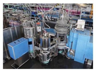
Figure 6: The fully polarized triple axis spectrometer KOMPASS and the CryoPad installed on the sample table.
