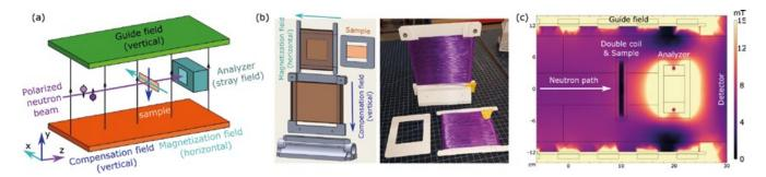
Figure 1: (a) Sketch of the relevant components in the experimental setup. The double-coil-setup has been omitted, showing only the additional fields created by it. (b) 3D-design and photo of the double-coil-setup. The sample, inner coil and outer coil form a nested compact sample environment with easy access to the sample. (c) Magnetic field distribution as calculated using COMSOL with fully compensated guide field.
