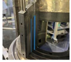
Figure 3: Adaption of the monochromator shielding for LADIFF: one of the new shielding elements comprised of a sandwich structure of lead and polyethylene (blue).
