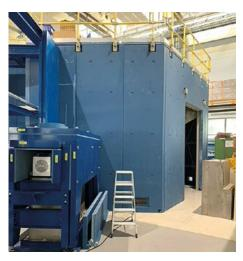
Figure 1: The instrument TOPAS: outer shielding and the chopper system (front) in the neutron Guide Hall East.
