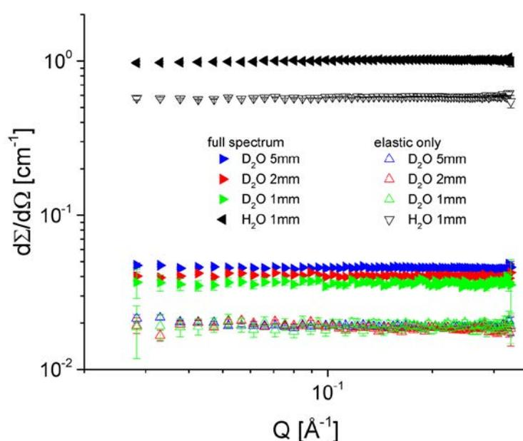
Fig. 2: The measured scattering cross section of H<sub>2</sub>O and D<sub>2</sub>O when full scattering spectrum or only the elastic scattering are considered.
