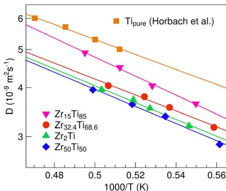
Fig. 4: Self-diffusion coefficients of Ti in Zr-Ti melts, measured using electromagnetic levitation at TOFTOF.
