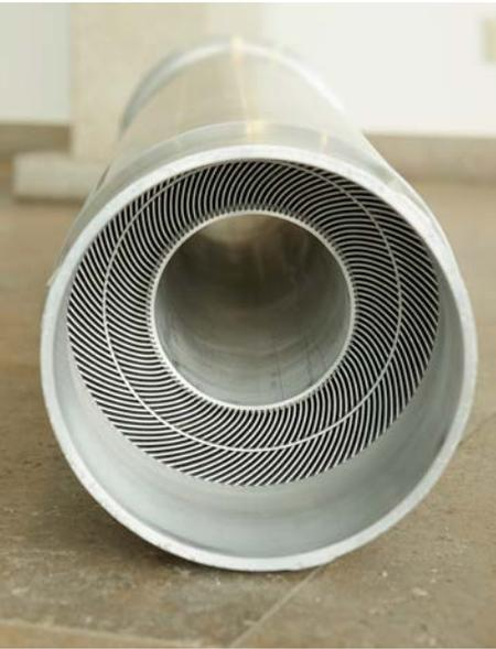
The fuel element of the FRM II is a hollow cylinder of some 1.3 m in length, 24 cm diameter and with a total weight of 53 kg. It contains approximately 8.1 kg of uranium enriched to 93 % of the fissile uranium  $^{235}\text{U}$ . The fuel in use is  $\text{U}_3\text{Si}_2$  dispersed in Al.
