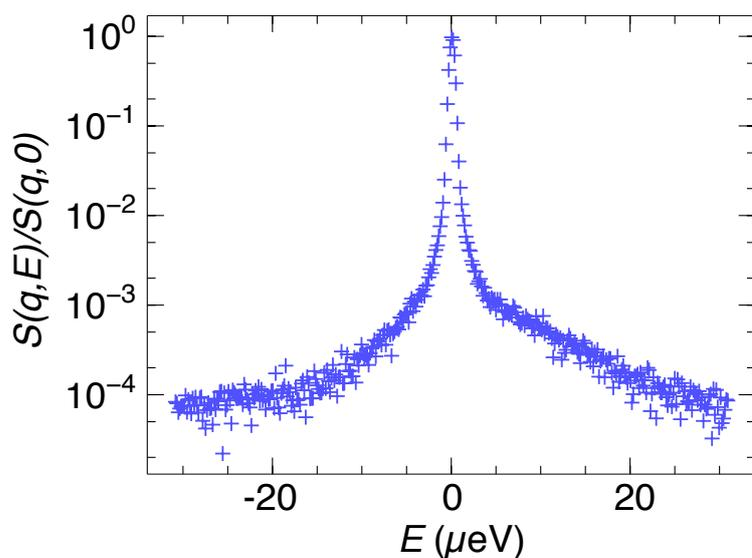
Fig. 2: Resolution function for a polymer sample for the high signal-to-noise set-up.
