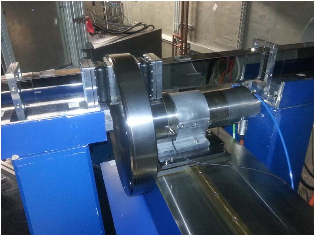
Fig. 1: The new focussing neutron guide with the background chopper.
