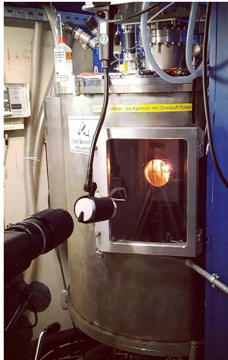
Fig. 2: Electromagnetic levitator (EML) of DLR installed at TOFTOF.
