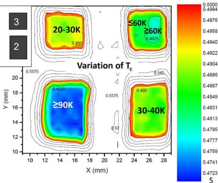
Fig. 2: 2D-S-parameter map of four 200 nm thin YBCO samples obtained by spatially resolved DBS (positron energy: 4 keV). The variation of the S-parameter (colour code, right) allows the determination of the local  $T_c$  inside the individual samples.
