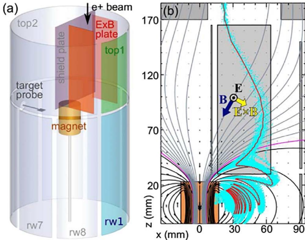
Fig. 4: (a) The experiment set-up for confining a pair plasma. (b) A typical simulation of lossless  $E \times B$  transport from field lines connecting to the beam line (top) and into the confinement region. Points along the trajectories of 100 particles are projected onto the  $xz$  plane (cyan dots), as is a single trajectory (red line) [6].
