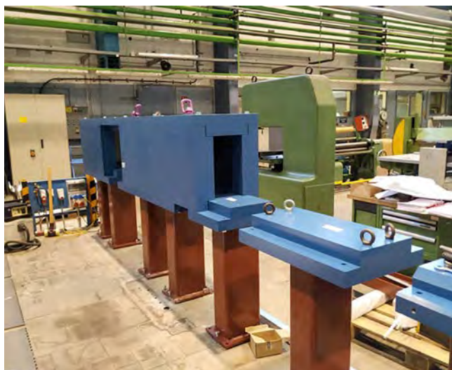
Figure 3: The shielding consists of 150 mm thick steel plates.
