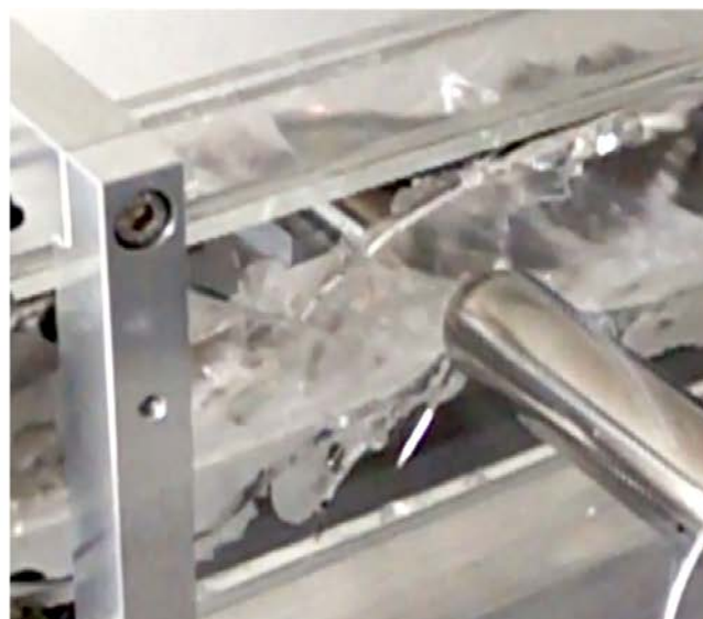
Figure 6: On the right-hand side standard neutron guide element with provoked implosion, on the left-hand side laminated glass guide element under equivalent conditions.
